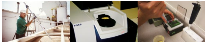
Bulk ingredients are sampled across the depth and length of the load and tested for macronutrients and mycotoxins
